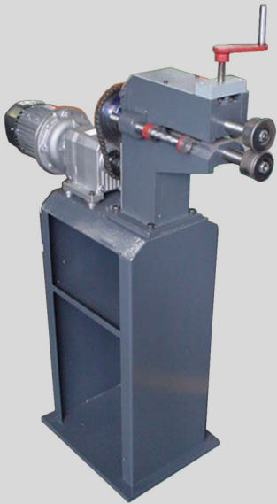
Jenny: • 1.6mm Capacity x 230mm From the side with 5 sets of wheels
